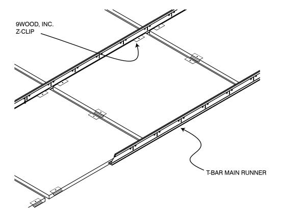
The 4100 Tegular Tile wood ceiling offers a tiled appearance. The 4100 Tegular Tile hangs from and is accented by 15/16" standard black T-Grid. Reveals between panels are created by the width of the T-Bar flange (i.e., 15/16").
