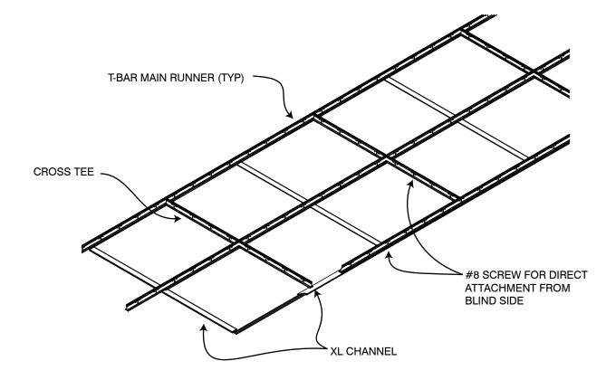
Designed with large wood panels in mind, the 4500 XL Channel Channel Tile wood ceiling offers a floating tiled appearance. The 4500 style installs progressively using perimeter extrusion clips (XL Channel). Minimum reveals are 3/8" typ., permitting a concealed suspension.
